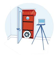
The doors, windows and envelope air-barrier materials must be in place at the time of the energy evaluation.
